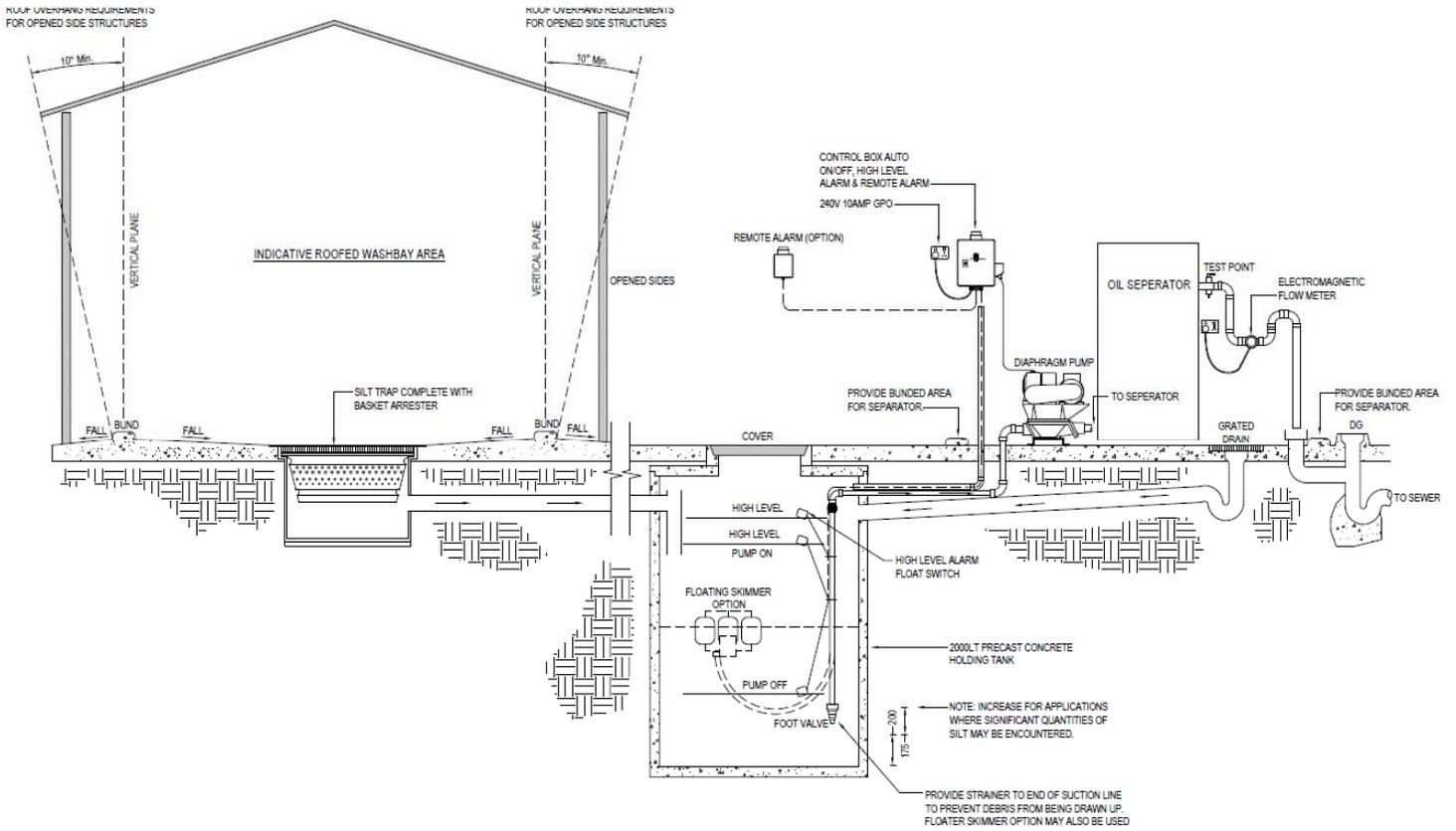
INDICATIVE ROOFED VEHICLE WASH BAY, HOLDING TANK AND OILS SEPARATOR DETAIL
